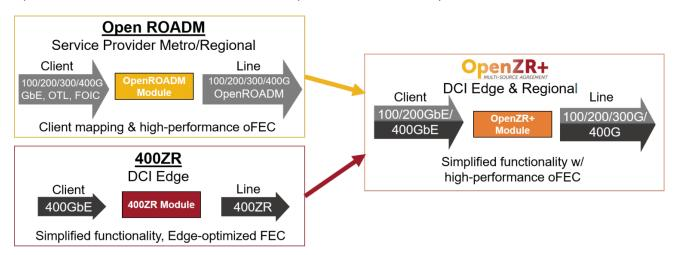
Specifically, 400G OpenZR+ combined the focus on ethernet traffic, higher performance, and multi-vendor interoperability to provide network operators with an operationally efficient solution for DCI and service provider applications with support for regional and long-haul reaches. Now the industry is looking to the OpenZR+ MSA group for guidance addressing similar applications with 800G coherent optical transceivers in small form-factor pluggable modules.
